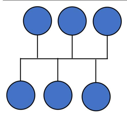
Bus topology uses a single cable which connects all the included nodes. The main cable acts as a spine for the entire network. One of the computers in the network acts as the computer server. When it has two endpoints, it is known as a linear bus topology.
