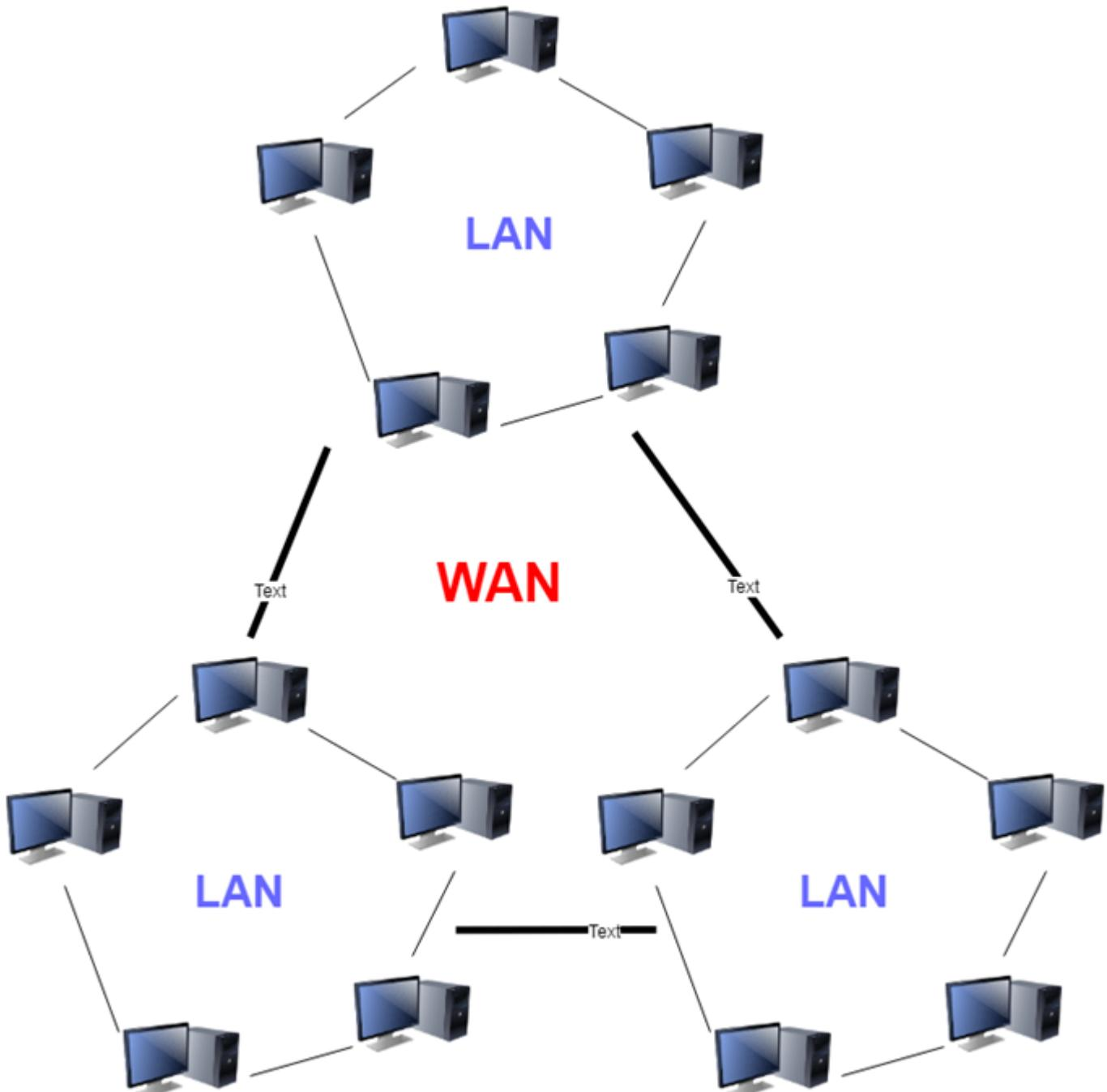
WAN (Wide Area Network) is another important computer network that which is spread across a large geographical area. WAN network system could be a connection of a LAN which connects with other LAN's using telephone lines and radio waves. It is mostly limited to an enterprise or an organization. Characteristics of LAN:
