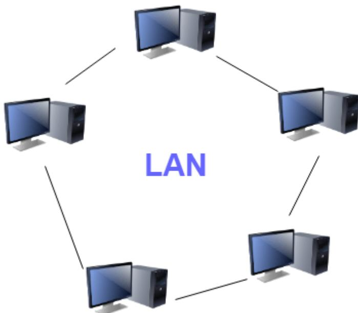
A Local Area Network (LAN) is a group of computer and peripheral devices which are connected in a limited area such as school, laboratory, home, and office building. It is a widely useful network for sharing resources like files, printers, games, and other application. The simplest type of LAN network is to connect computers and a printer in someone's home or office. In general, LAN will be used as one type of transmission medium.
