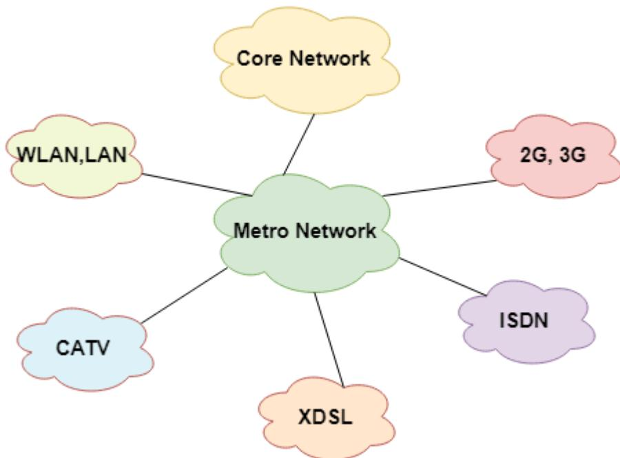
A Metropolitan Area Network or MAN is consisting of a computer network across an entire city, college campus, or a small region. This type of network is large than a LAN, which is mostly limited to a single building or site. Depending upon the type of configuration, this type of network allows you to cover an area from several miles to tens of miles.
