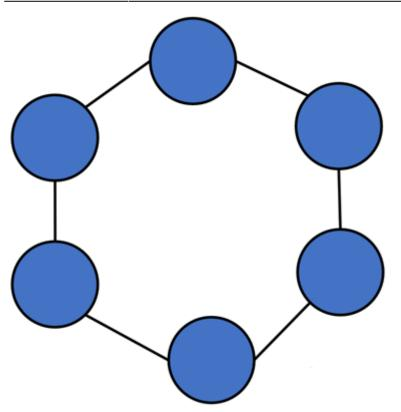
In a ring network, every device has exactly two neighboring devices for communication purpose. It is called a ring topology as its formation is like a ring. In this topology, every computer is connected to another computer. Here, the last node is combined with a first one.
