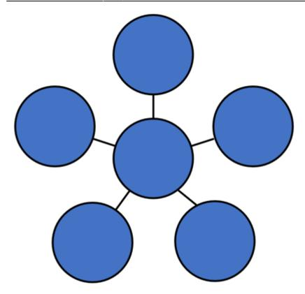
In the star topology, all the computers connect with the help of a hub. This cable is called a central node, and all other nodes are connected using this central node. It is most popular on LAN networks as they are inexpensive and easy to install.
