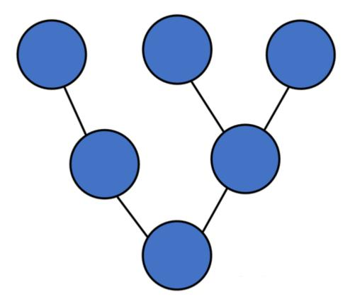
Tree topologies have a root node, and all other nodes are connected which form a hierarchy. So it is also known as hierarchical topology. This topology integrates various star topologies together in a single bus, so it is known as a Star Bus topology. Tree topology is a very common network which is similar to a bus and star topology.
