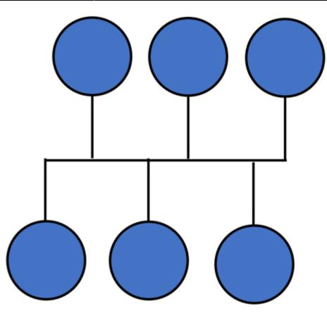
Bus topology uses a single cable which connects all the included nodes. The main cable acts as a spine for the entire network. One of the computers in the network acts as the computer server. When it has two endpoints, it is known as a linear bus topology.
